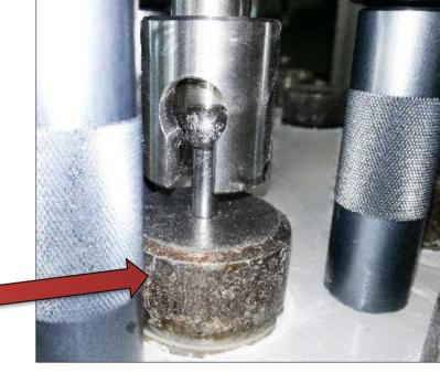
Figure 2. The view of: a) pull-off tests apparatus, b) steel disc glued to the surface
