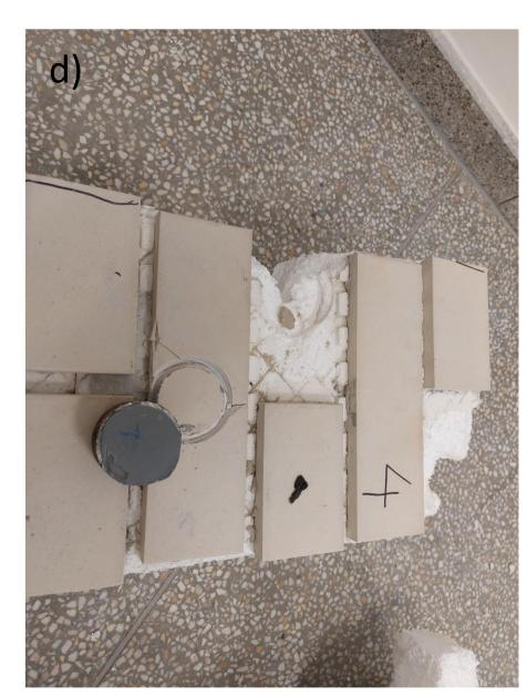
**Figure 3.** The view of: a) cohesive failure model in the insulation, b) adhesive failure model between the cladding and the glue, c) cohesive failure model inside the glued layer, d) adhesive failure between the steel disc and the cladding
